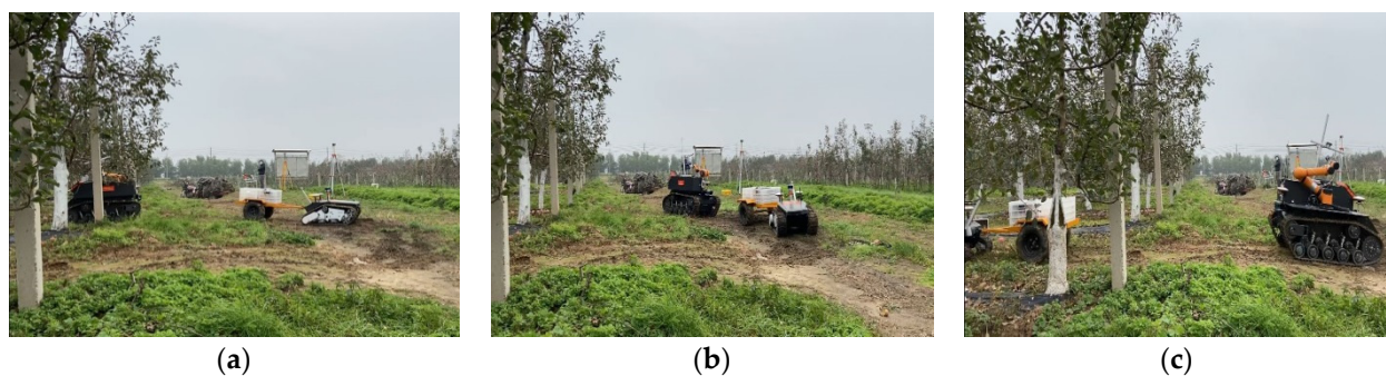
Figure 17. Picking and transporting robots carrying out autonomous navigation trials in an orchard. (a) Start turning at the head of the ground; (b) picking and transporting robots turn at the same time; (c) start of apple tree in-row navigation.
