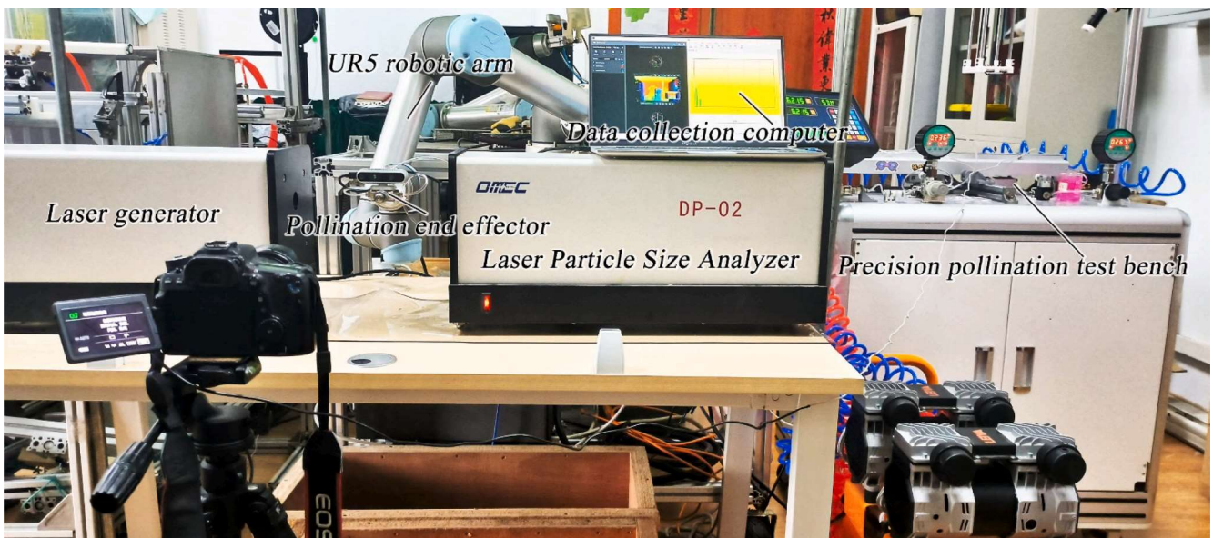
Fig. 11. Experimental setup for droplet size distribution detection.
